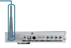
Note: You may have an Ethernet cable plugged into the unit and have the wireless antenna connected. Neither will interfere with the other, but only one network can be accessed at a time (wired or wireless). The network connection type is selected in the Setup Wizard and can be changed by going to the Setup Menu. To access the Setup Menu, press the SETUP button on the remote control.
