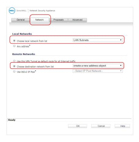
Configure a new address object to define the IP address of the remote range reachable through the VPN with the DSR-1000AC.
