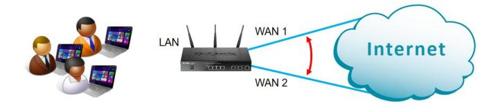
Using two Internet connections allows to increase total available bandwidth and at the same time offer fault tolerance.
