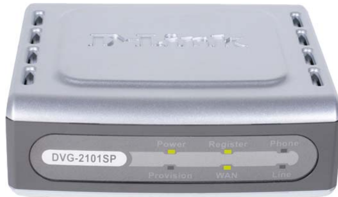
DVG-2101SP LEDs showing a successful registration to the VoIP Provider
