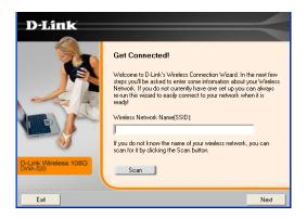
Click the Scan button to display a list of wireless networks (site survey). Click on the network name (SSID) and click **Next**.
