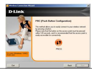
Note: please press the button on the access point within 120 seconds and it is recommended that the access point is nearby.
