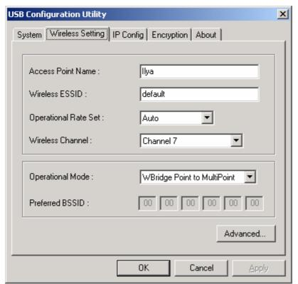
Notice that no BSSID is required for this setting. The same also applies to "Access point" mode.
