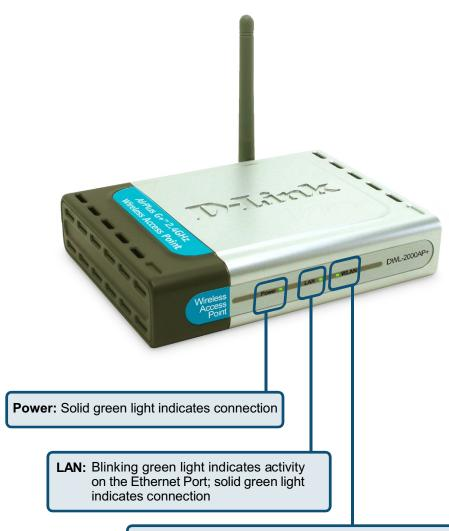
**WLAN:** Blinking green light indicates wireless activity; solid green light indicates connection
