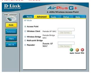
The DWL-2000AP+ can be configured to perform in any of four modes: a Wireless Access Point; a Wireless Client; a Wireless Bridge; or a Multi-Point Bridge.
