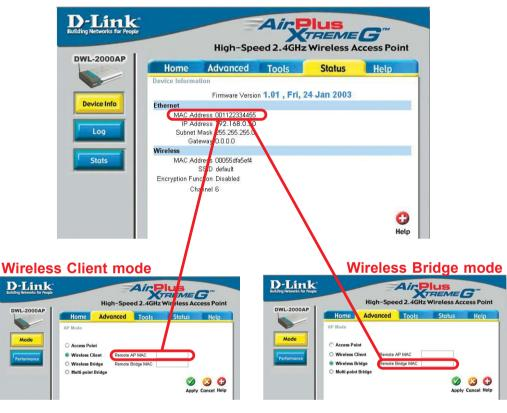
When using the DWL-2000AP in **Wireless Client** mode, you will enter the MAC address of the Remote AP.
