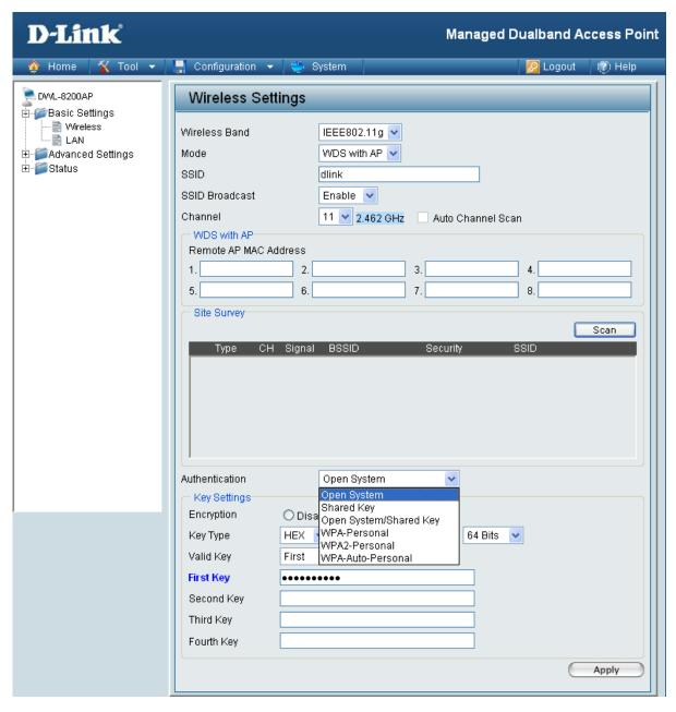
In WDS with AP mode, the **DWL-8200AP** wirelessly connects multiple networks, while still functioning as a wireless AP.
