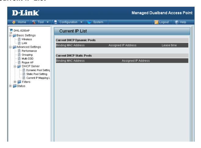
This screen displays information about the current DHCP dynamic and static IP address pools. This information is available when you enable the DHCP function of the **DWL-8200AP** and assign dynamic and static IP address pools.
