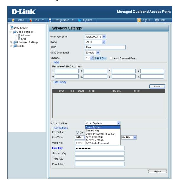
In WDS, the **DWL-8200AP** wirelessly connects multiple networks, without functioning as a wireless AP.
