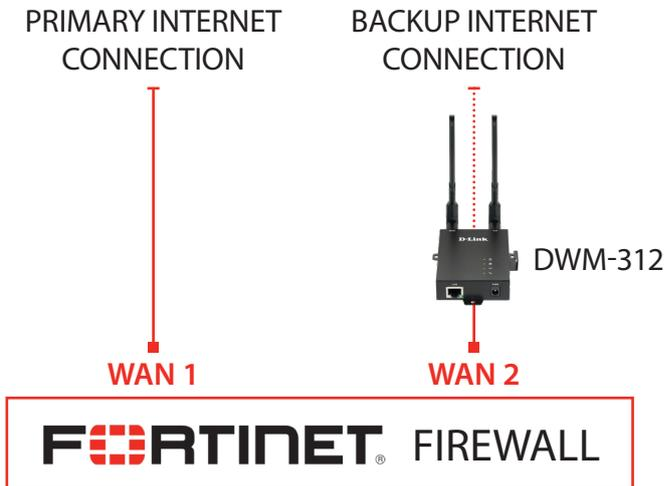
**STEP 1.** To set the DWM-312 4G LTE Modem in Bridge Mode, connect it to your computer and log into it via <http://192.168.0.1>.
