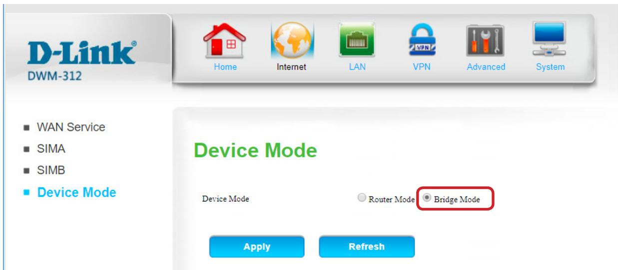
The screenshot shows the D-Link DWM-312 web interface. The top navigation bar includes Home, Internet, LAN, VPN, Advanced, and System. The left sidebar lists WAN Service, SIMA, SIMB, Device Mode, and Router Mode (highlighted). The main content area is titled "Device Mode" and shows the "Device Mode" section. The "Bridge Mode" radio button is selected and highlighted with a red box. Below it are "Apply" and "Refresh" buttons, with the "Apply" button highlighted with a red box.
