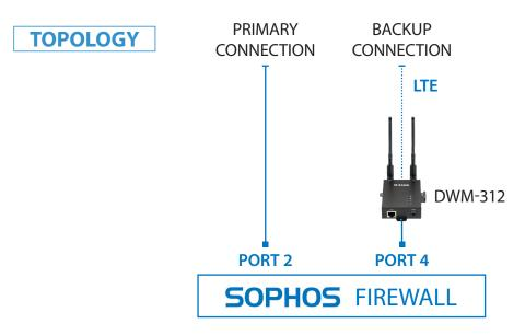
**STEP 1.** To set the DWM-312 4G LTE Modem in Bridge Mode, connect it to your computer and log into it via http://192.168.0.1.
