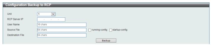
Figure 13-17 Configuration Backup to RCP Window
