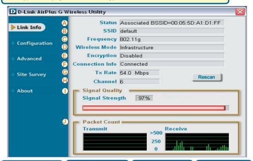
F. Connection Info: Displays connected or authenticated information. G. TxRate: The default setting is Auto; meaning, TxRate settings are automatically determined by the DWL-G122 depending on the distance from the access point.
