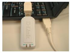
B. Insert one end of the USB Adapter into the provided USB cable and plug the other end into your computer's USB Port. 3
