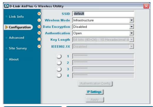
N. Authentication: You can specify the authentication mode for the wireless network. The default setting is set to Open Authentication.
