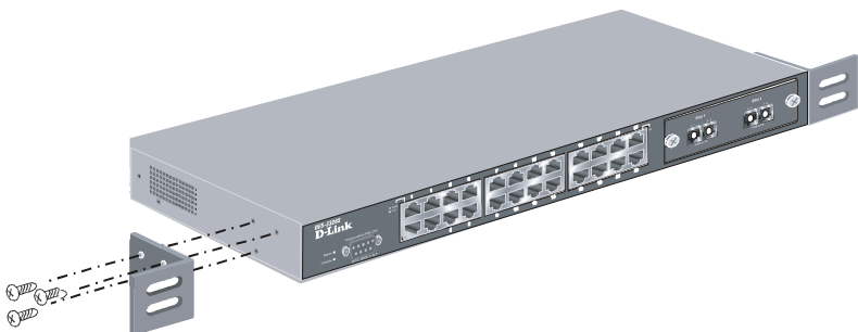
Figure 2- 2. Attaching the mounting brackets to the switch
