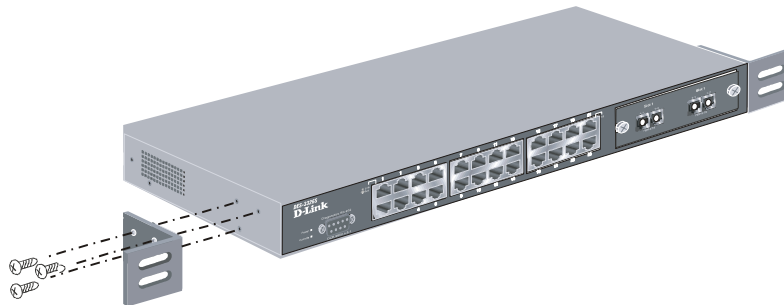
Figure 2-2. Attaching the mounting brackets to the switch
