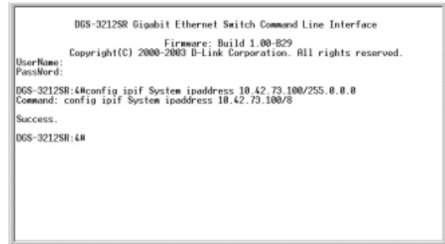
Figure 1-3. Assigning the Switch an IP Address
