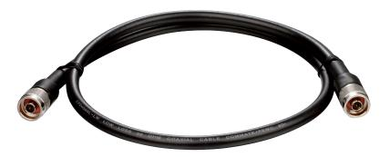
D-Link's ANT70-CB1N and ANT70-CB1RN are one-meter extension cables that connect D-Link outdoor antennas to D-Link outdoor access points. The ANT70-CB1N connects an N plug to an N plug while the ANT70-CB1RN connects a RP-N plug to an N plug. The cables can transmit data with low loss at both 2.4 GHz and 5 GHz. Both cables are certified with the IP67 standard, meaning they are waterproof and dustproof, allowing them to function well in adverse outdoor environments.
