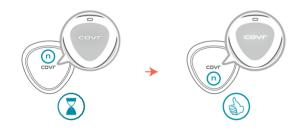
Wait for the COVR LED on the new unit to light up solid white. When it does, the device is paired and ready to use.
