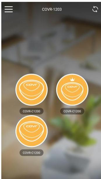
The device icon with a crown sign indicates the COVR Router.
