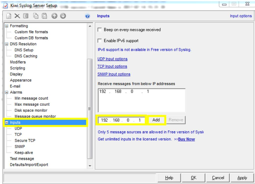
**Step 3:** Enable "Enable Logging to Syslog Server", and fill in the IP address of the PC that has the Kiwi Syslog Server installed on it:
