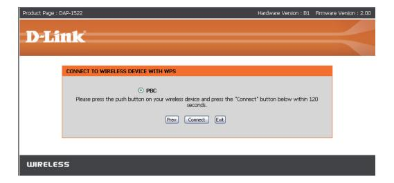
Press down the WPS Button on the wireless device you are adding to your network to complete the setup.
