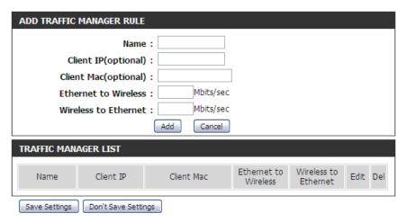
**Note:** Normally the wireless connection transmits application data packets based on the wireless to Ethernet speed and Ethernet to wireless speed. Users can treat the two speeds as system transmission bandwidth, where all applications will share the whole system bandwidth based on assigned priorities. Note that the maximum amount of bandwidth that can be used is the same as the set value of both speeds.
