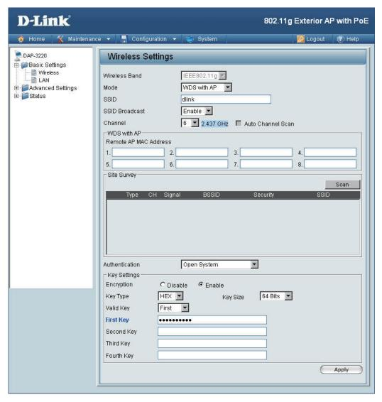
In WDS with AP mode, the DAP-3220 wirelessly connects multiple networks while still functioning as a wireless AP.
