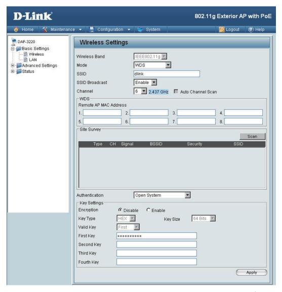
In WDS mode, the DAP-3220 wirelessly connects multiple networks, without functioning as a wireless AP.
