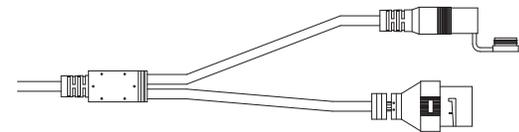
**If you are using a power adapter (not included) to power your camera, wind waterproof tape around the connection in an overlapping manner to cover it.**
