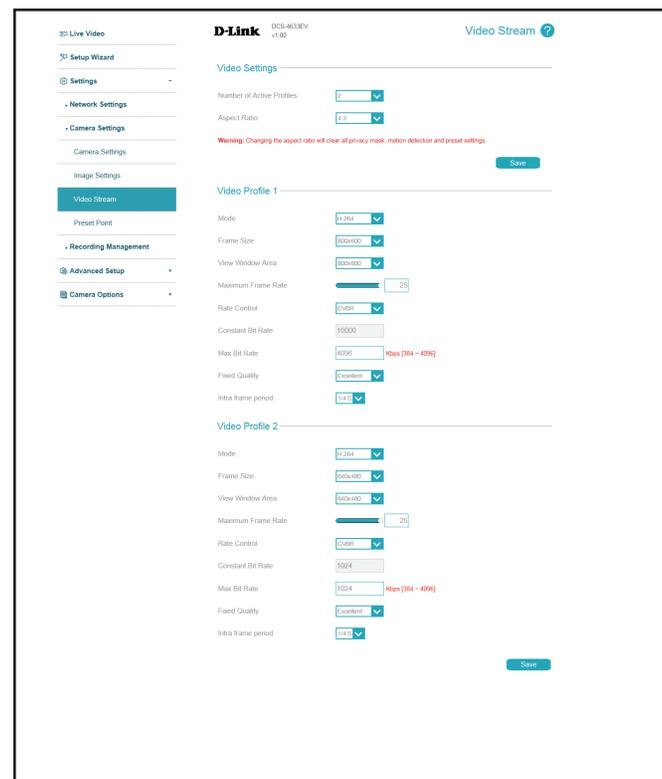
**Constant Bit Rate:** If the **Rate Control** is set to **CBR**, you can set the bit rate to use for this video profile.
