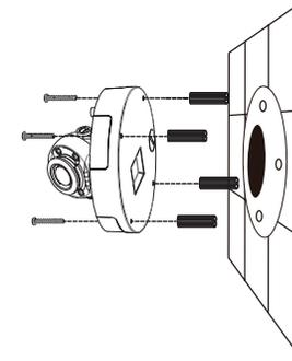
**If you are mounting the camera to the ceiling,** use a flathead screwdriver to remove the plastic hole cover from the bottom of the base, then guide the cables through the bottom.
