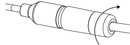
**If you are using PoE to power your camera,** use the power connector cap to seal the power connector.
