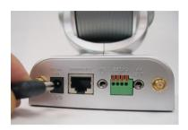
When you have a proper connection, the **LED** (Light Emitting Diode) on the front of the camera will change from red to green. The light may blink on and off and your computer may show an intermittant loss of connectivity, this is normal until you have configured your camera.
