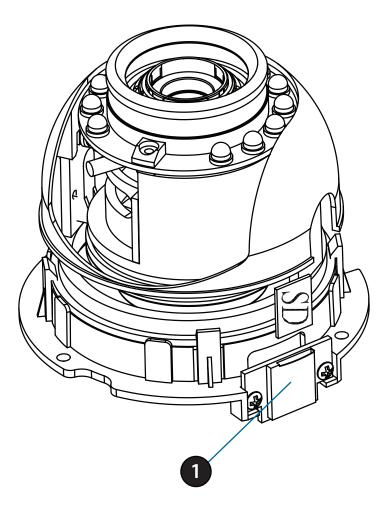
1 Micro SD Card Slot Insert a Micro SD card for Local storage for storing recorded image and video
