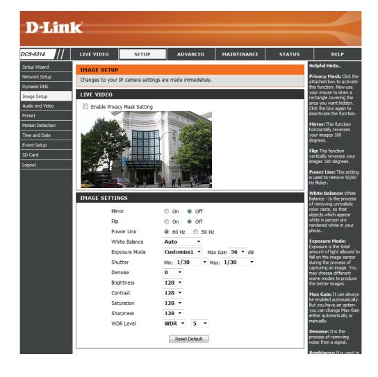
Exposure box to set the camera for Indoor, Outdoor, or Mode: Night environments, or to Moving to capture moving objects. The Low Noise option will focus on creating a high-quality picture without noise. You can also create 3 different custom exposure modes. The Max Gain setting will allow you to control the maximum amount of gain to apply to brighten the picture.
