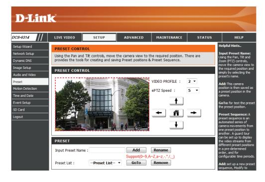
**Preset** This section allows you to create a preset sequence, **Sequence:** which automatically moves the camera's view between a set of preset views.
