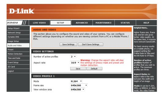
Maximum A higher frame rate provides smoother motion frame rate: for videos, and requires more bandwidth. Lower frame rates will result in stuttering motion, and requires less bandwidth.
