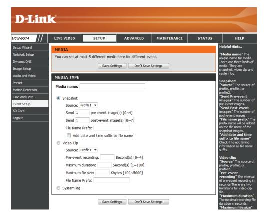
Add date and Check this to add timing information as file name suffix. Please see the previous page for an example on how the file name will be time suffix to determined if this option is enabled.
