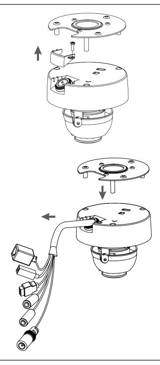
Reattach the top part of the camera housing, and secure it by tightening the three retaining screws.
