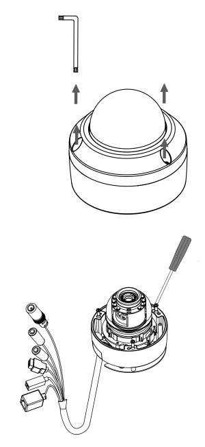
Remove the mounting plate from the lower half of the camera housing. It can now be attached to a wall or ceiling using the mounting guide. Please see "Deploying the Camera" on page 13 for more instructions.
