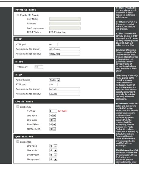
Enable IPv6: Enable the IPv6 setting to use the IPv6 protocol. Enabling the option allows you to manually set up the address, specify an optional IP address, specify an optional router and an optional primary DNS.
