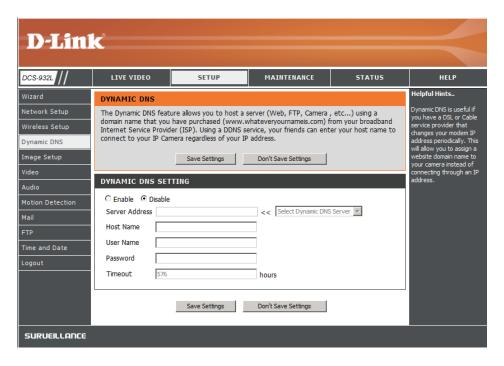
**DDNS:** (Dynamic Domain Name Server) will hold a DNS host name and synchronize the public IP address of the modem when it has been modified. The username and password are required when using the DDNS service.
