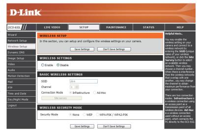
**Wireless Security** For security, there are three choices; **None**, **WEP**, and **WPA-PSK** / **WPA2-PSK**. Select the same encryption method that is being used by **Mode:** your wireless device/ router.
