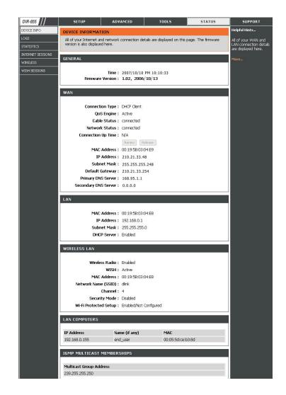
**Note:** Because a dynamic WAN IP can change from time to time depending on your ISP, you may want to obtain a Static IP address from your ISP. A Static IP address is a fixed IP address that will not change over time and will be more convenient for you to use to access your camera from a remote location. The Static IP Address will also allow you to access your camera attached to your router over the Internet.
