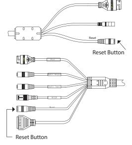
If your camera model does not have the multi-head cable, the Reset Button is located behind the cover.
