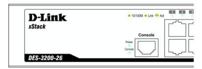
Figure 1-6. LED Indicators on DES-3200-26 Ver. B1 Switch
