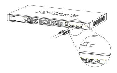
Figure 1- 4. Inserting the Mini-GBIC modules into the Switch (DES-3200-28 Ver. B1)
