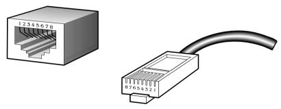
Figure B- 1. The standard RJ-45 port and connector
