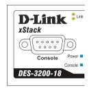
Figure 1-3. LED Indicators on DES-3200-18 Ver. A1 Switch
