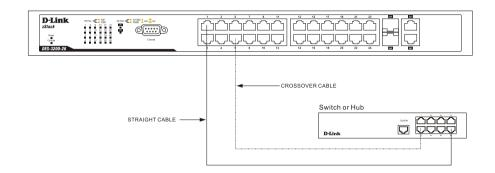
Figure 3- 3. Switch connected to a normal (non-Uplink) port on a hub or switch using a straight or crossover cable
