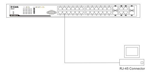
Figure 3-1. DES-3200-28 Ver. A1 connected to an end node
