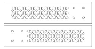
Figure 1-20. Side panels of the DES-3200-10 Ver. A1 and DES-3200-18 Ver. A1
