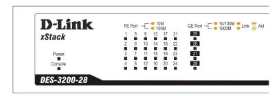
Figure 1-7. LED Indicators on DES-3200-28 Ver. A1 Switch
