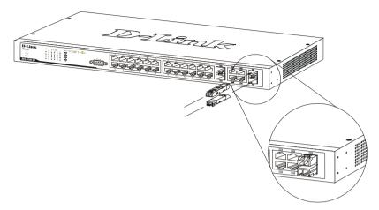
Figure 1-25. Inserting the Mini-GBIC modules into the Switch (DES-3200-28 Ver. A1)
