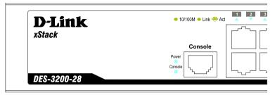
Figure 1-8. LED Indicators on DES-3200-28 Ver. B1 Switch
