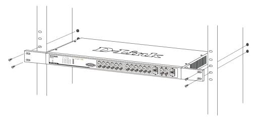
Figure 2-2. Installing Switch in a rack
