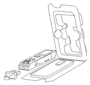
Figure 1-27. Installing the Mini-GBIC Module
