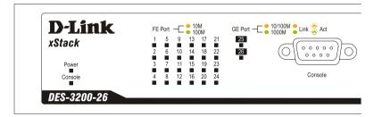
Figure 1-5. LED Indicators on DES-3200-26 Ver. A1 Switch
