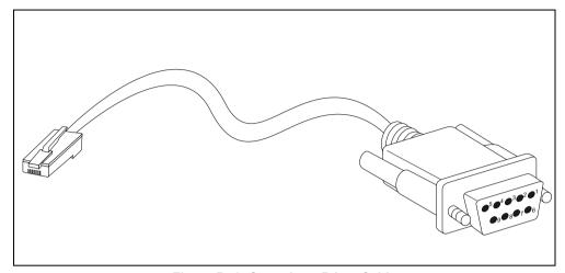
Figure B- 2. Console-to-RJ-45 Cable
