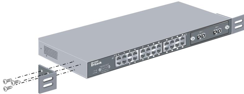
**Figure 2- 2. Attaching the mounting brackets to the switch**
