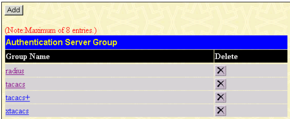
Figure 11- 17. Authentication Server Group Settings window
