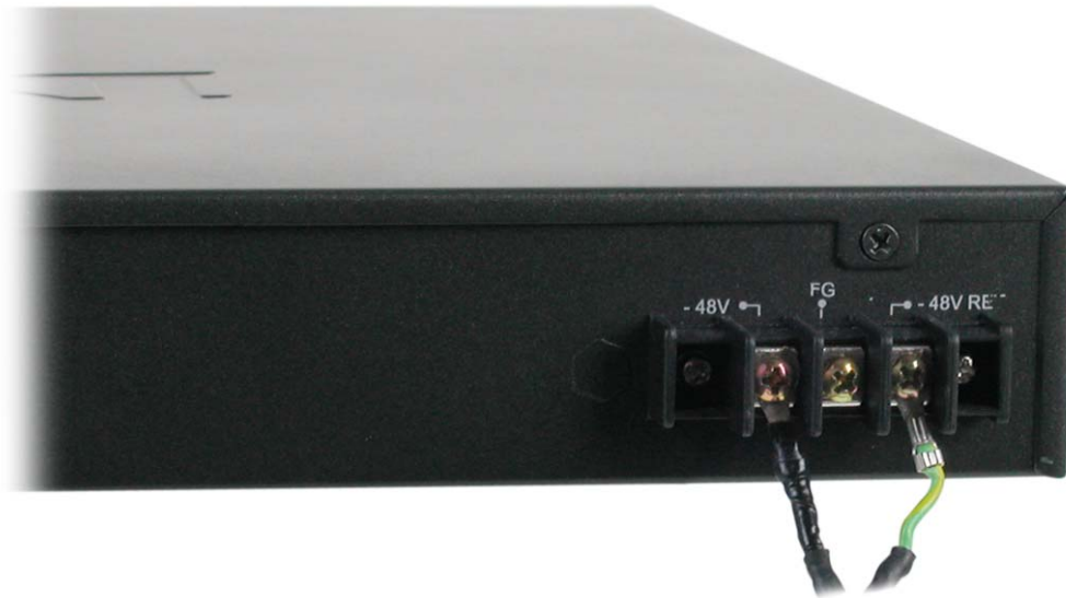
Figure 2 - 4. Power connections attached to contacts on assembly
