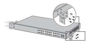
Align the brackets and rack holes. Fasten each bracket to the rack.
