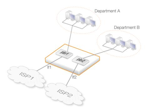
Figure 4.8. Virtual Routing
