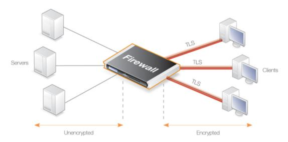
Figure 6.7. TLS Termination
