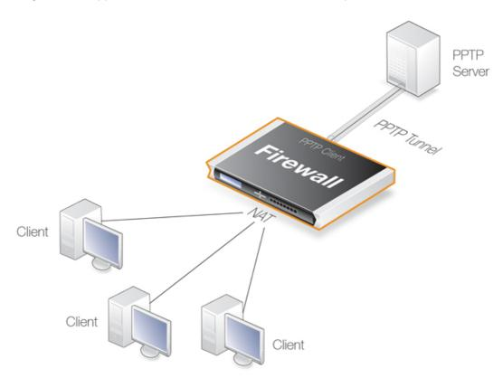
Figure 9.3. PPTP Client Usage
