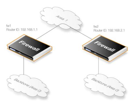
Figure 4.12. Virtual Links with Partitioned Backbone
