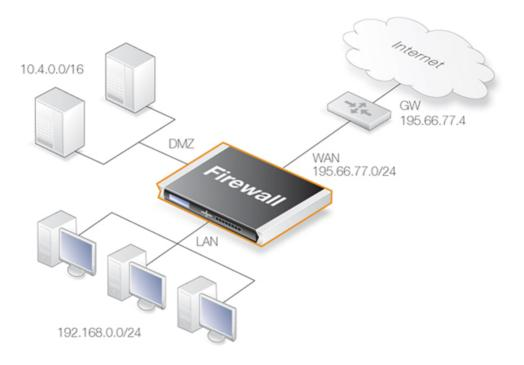
Figure 4.1. A Typical Routing Scenario
