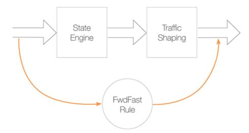
Figure 10.2. FwdFast Rules Bypass Traffic Shaping
