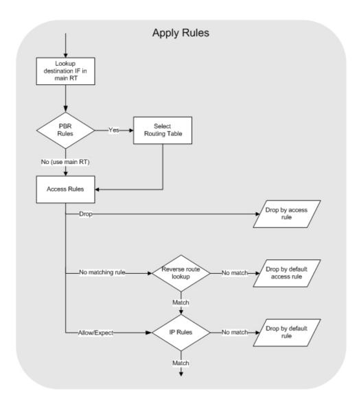
Figure 1.4. Expanded Apply Rules Logic
