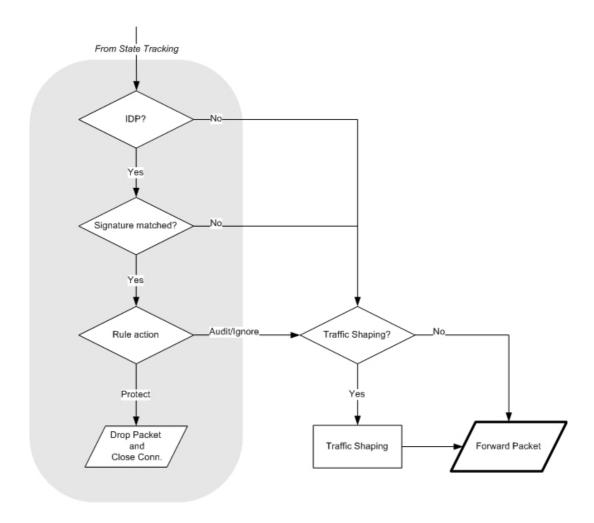
Figure 1.3. Packet Flow Schematic Part III
