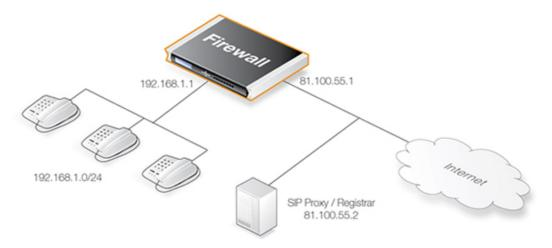
The SIP proxy in the above diagram could alternatively be located remotely across the Internet. The proxy should be configured with the **Record-Route** feature enabled to insure all SIP traffic to and from the office clients will be sent through the SIP Proxy. This is recommended since the attack surface is minimized by allowing only SIP signaling from the SIP Proxy to enter the local network.
