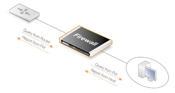
Figure 4.19. Multicast Proxy Mode
