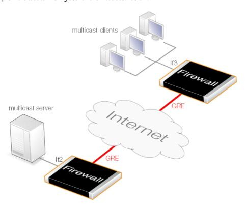
Figure 4.20. Tunneling Multicast using GRE
