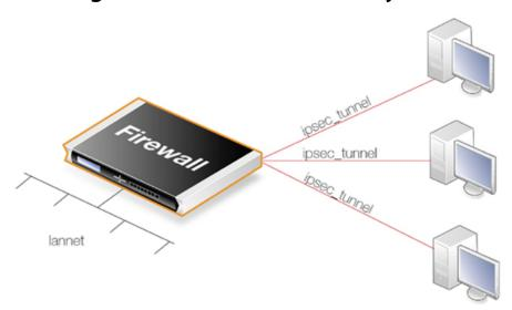
This section details the setup with roaming clients connecting through an IPsec tunnel using pre-shared keys to a protected **Local Network** which is located behind a NetDefend Firewall.
