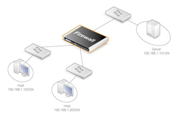
Figure 4.25. An Example BPDU Relaying Scenario
