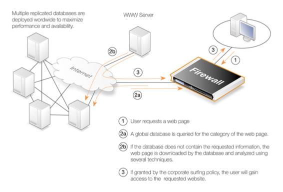
Figure 6.8. Dynamic Web Content Filtering Flow
