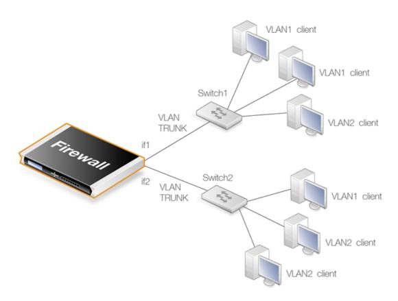
Figure 3.2. VLAN Connections
