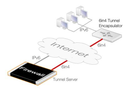
Figure 3.5. Acting as a 6in4 Tunnel Server
