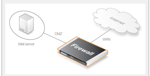
An IDP rule called IDPMailSrvRule will be created, and the Service object to use is the SMTP service. The Source Interface and Source Network defines where traffic is coming from, in this example the external network. The Destination Interface and Destination Network define where traffic is directed to, in this case the mail server. The Destination Network should therefore be set to the object defining the mail server.
