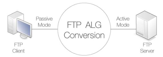
Figure 6.3. FTP ALG Hybrid Mode
