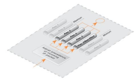
Figure 10.5. Minimum and Maximum Pipe Precedence
