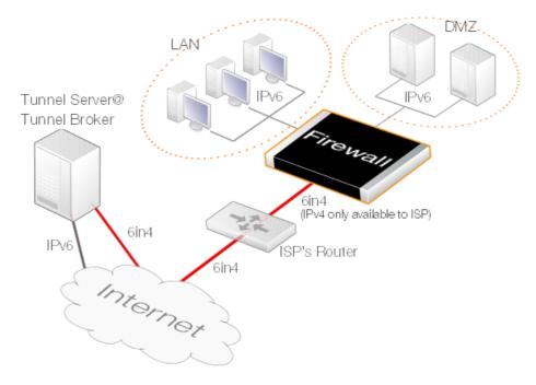
Figure 3.4. IP6in4 Tunnel Usage
