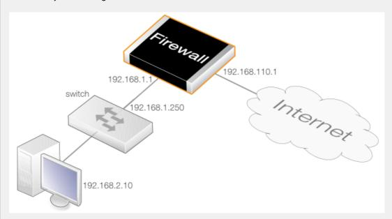
An HTTP threshold of 10 connections/second is to be applied to traffic. If the connection rate exceeds this, NetDefendOS will instruct the switch to block the host (within the network range 192.168.2.0/24).
