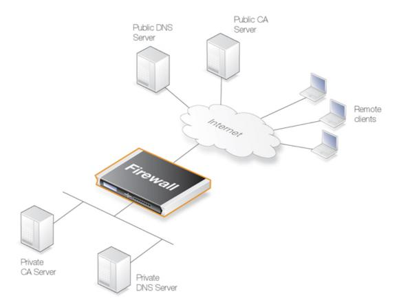
**Figure 9.8. Certificate Validation Components**
