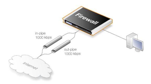
Figure 10.7. A Basic Traffic Shaping Scenario
