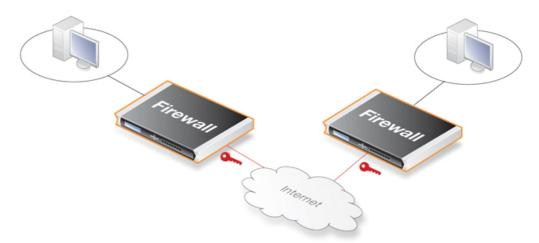
2. **Client to LAN connection** - Where many remote clients need to connect to an internal network over the Internet. In this case, the internal network is protected by the NetDefend Firewall to which the client connects and the VPN tunnel is set up between them.
