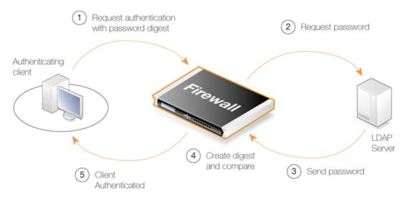
Figure 8.2. LDAP for PPP with CHAP, MS-CHAPv1 or MS-CHAPv2
