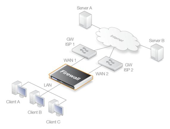
Figure 4.7. A Route Load Balancing Scenario
