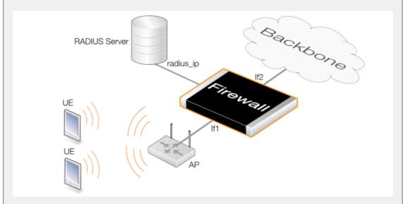
After successful authentication, IP address leases will be handed out by a DHCP server object called *rr\_dhcp\_server*. It is assumed the UEs will be allocated addresses belonging to the network 192.168.10.10-192.168.10.255 that will be defined in an IPv4 address object called *client\_net*.
