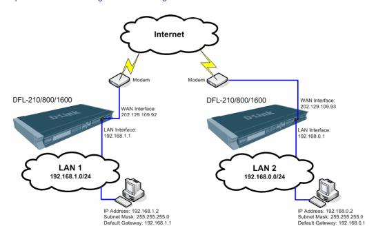
In our example the IPSec VPN tunnel is established between two LANs: 192.168.0.x and 192.168.1.x. **NOTE: It is essential to have private networks (LAN 1 and LAN 2) on different subnets.**
