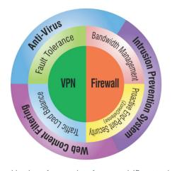
combination of users, interfaces, and IP networks. The firewall can actively handle Internet content in both regular HTTP and secured HTTPS by stripping potential malicious objects, such as Java Applets, JavaScripts/VBScripts, ActiveX objects, and cookies. Integration of SafeSearch Enforcement also ensures that results from search engine providers are provided without malicious content.
