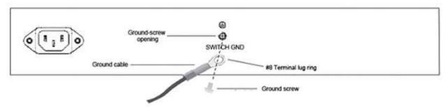
Figure 12 –Ground cable, screw and #8 terminal lug ring
