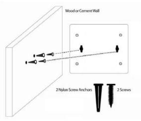
Figure 10 – Wall mount installation
