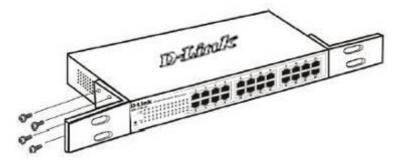
Figure 3-2 – Attach the mounting brackets to the Switch
