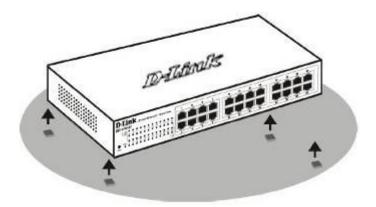
Figure 3-1 – Attach the adhesive rubber pads to the bottom
