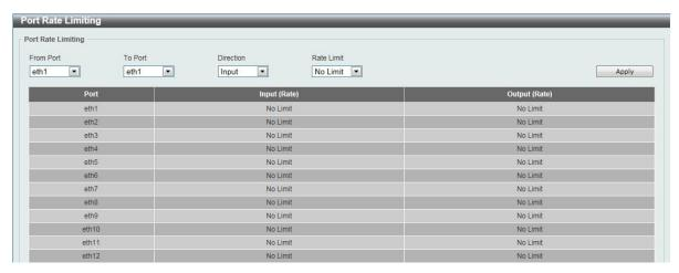
Figure 8-2 Port Rate Limiting window
