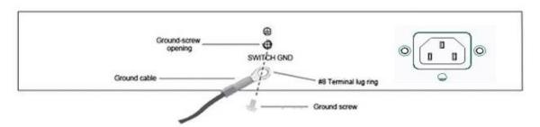
Figure 3-5 - Ground cable, screw and #8 terminal lug rings
