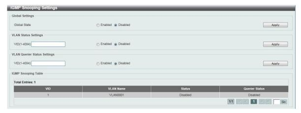
Figure 7-28 IGMP Snooping Settings window
