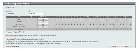
Figure 7-7 VLAN Configuration Wizard window
