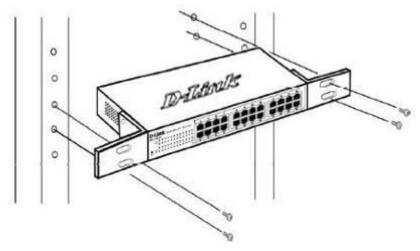
Figure 3-3- Mount the Switch in the rack or chassis
