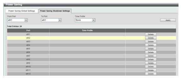
Figure 12-2 Power Saving Shutdown Settings window
