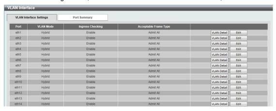
Figure 7-11 VLAN Interface window
