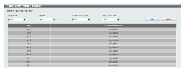
Figure 9-2 Traffic Segmentation Settings window
