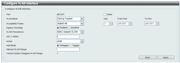
Figure 5-20 VLAN Interface (802.1Q-Tunnel) Window
