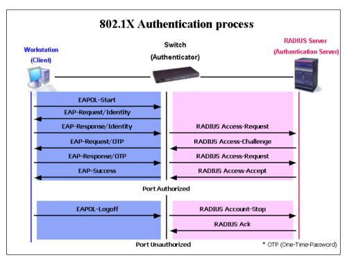
Figure 9-9 The 802.1X Authentication Process
