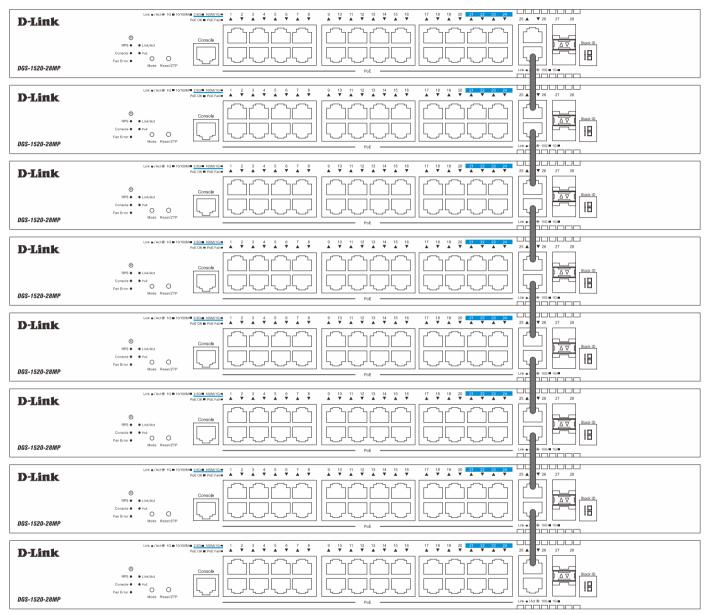
Figure 4-84 Duplex Chain Stacking Topology
