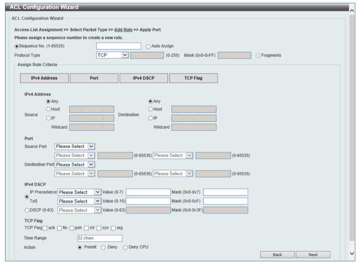
Figure 8-6 ACL Configuration Wizard (Extended IPv4 ACL) Window
