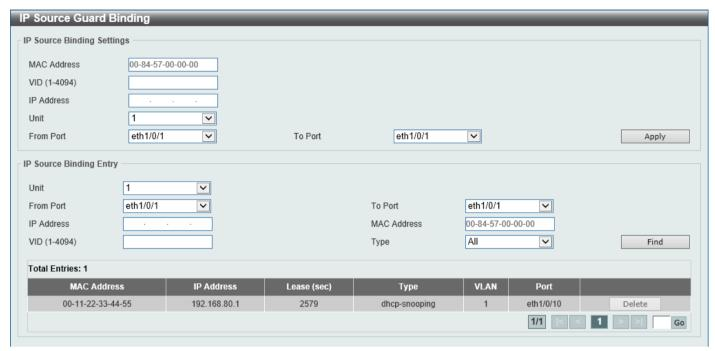
Figure 9-52 IP Source Guard Binding Window
