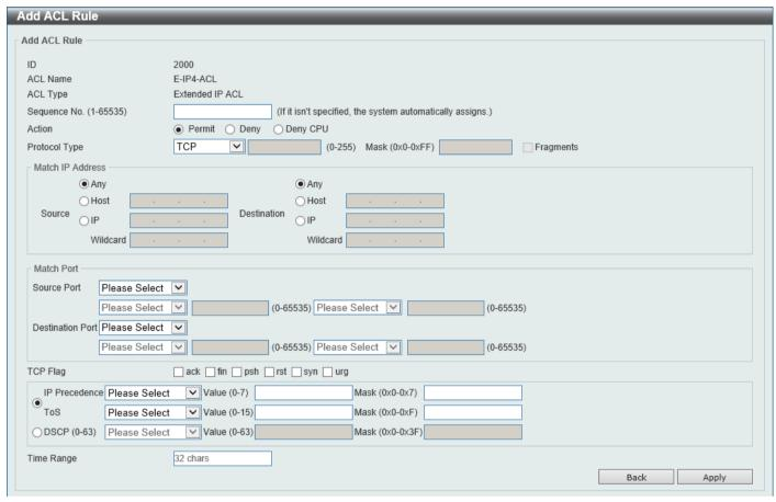
Figure 8-15 Extended IP ACL (Add Rule) Window
