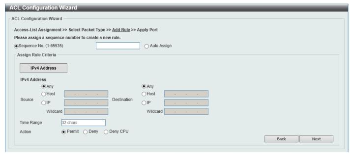
Figure 8-5 ACL Configuration Wizard (Standard IPv4 ACL) Window
