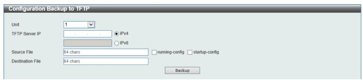
Figure 13-12 Configuration Backup to TFTP Window
