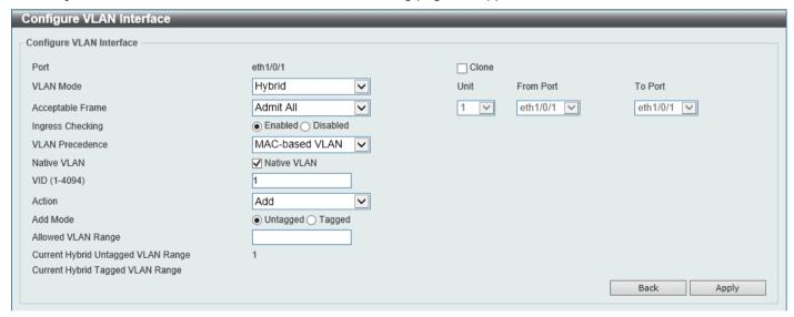
Figure 5-18 VLAN Interface (Hybrid) Window
