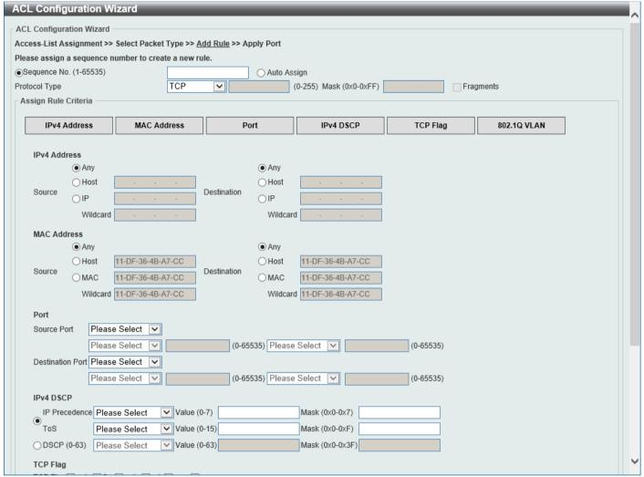
Figure 8-9 ACL Configuration Wizard (Extended Expert ACL) Window
