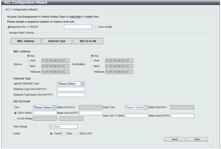
Figure 8-4 ACL Configuration Wizard (Extended MAC ACL) Window
