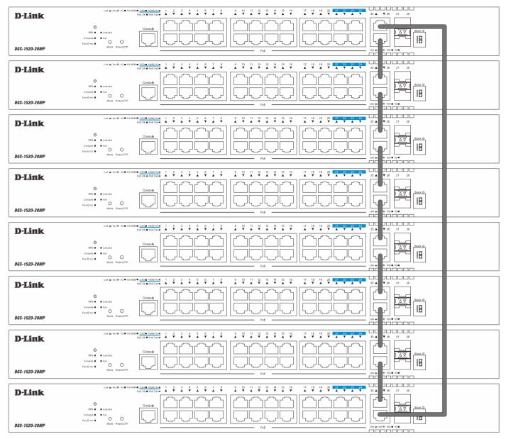
Figure 4-85 Duplex Ring Stacking Topology
