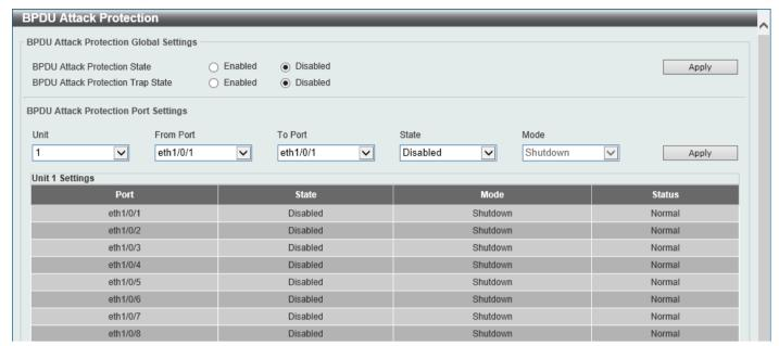
Figure 9-71 BPDU Attack Protection Window
