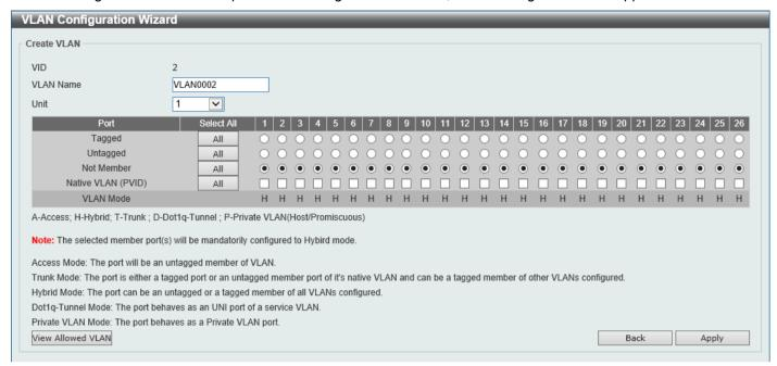
Figure 5-10 VLAN Configuration Wizard (Create VLAN) Window
