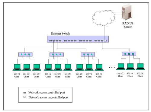
Figure 9-11 Example of Typical Host-based Configuration
