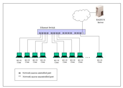
Figure 9-10 Example of Typical Port-based Configuration
