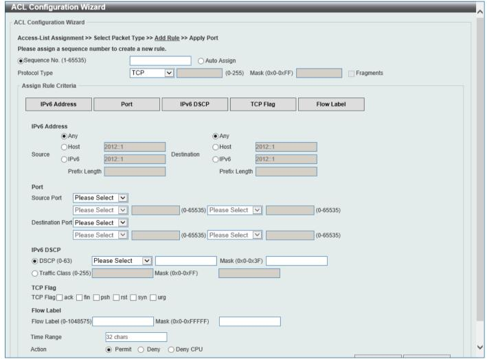
Figure 8-8 ACL Configuration Wizard (Extended IPv6 ACL) Window
