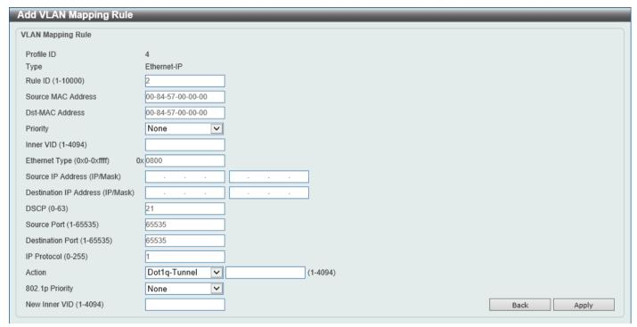
Figure 5-53 VLAN Mapping Profile (Ethernet-IP, Add Rule) Window
