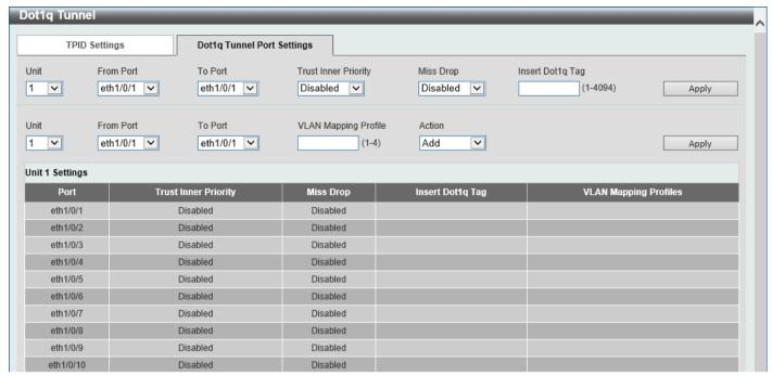
Figure 5-47 Dot1q Tunnel Settings (Dot1q Tunnel Port Settings) Window
