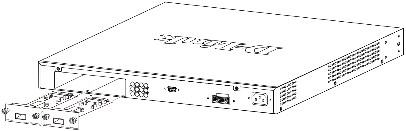
Figure 2- 18. Inserting the optional module into the Switch (DGS-3450)
