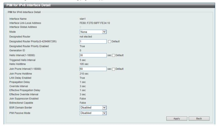
Figure 6-126 PIM for IPv6 Interface (Edit) Window
