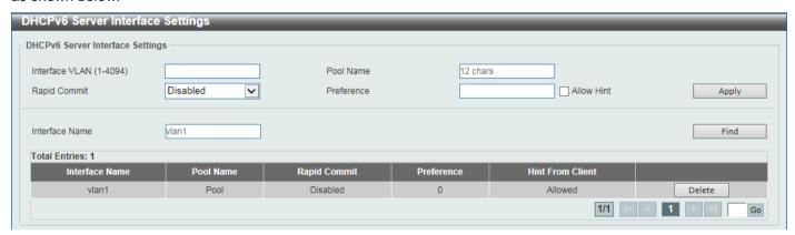
Figure 4-47 DHCPv6 Server Interface Settings Window
