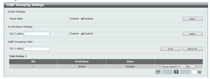
Figure 5-75 IGMP Snooping Settings Window
