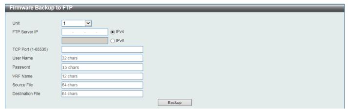
Figure 16-9 Firmware Backup to FTP Window
