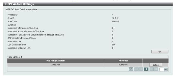
Figure 6-77 OSPFv3 Area Settings (Process ID, Normal) Window
