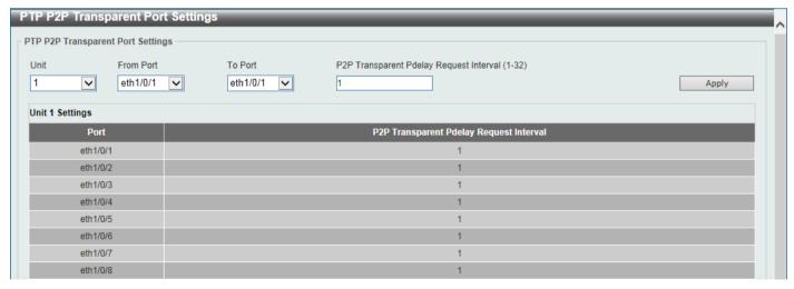
Figure 3-32 PTP P2P Transparent Port Settings Window
