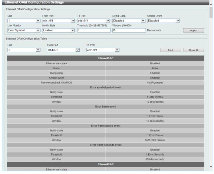
Figure 10-23 Ethernet OAM Configuration Settings Window
