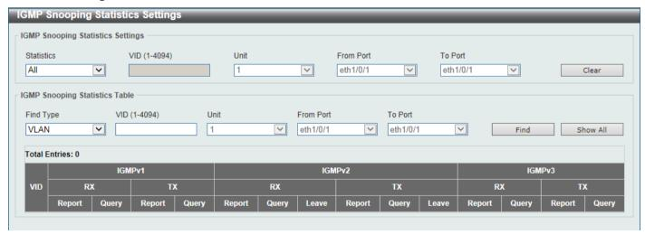
Figure 5-84 IGMP Snooping Statistics Settings Window
