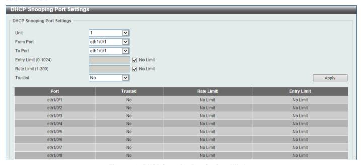
Figure 9-42 DHCP Snooping Port Settings Window
