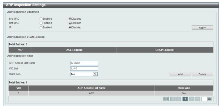
Figure 9-48 ARP Inspection Settings Window
