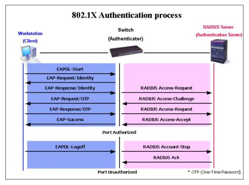
Figure 9-9 The 802.1X Authentication Process
