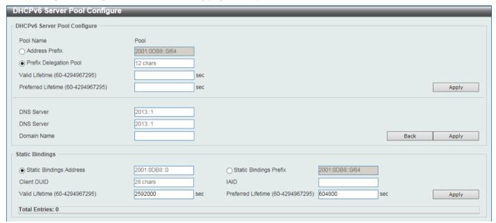
Figure 4-43 DHCPv6 Server Pool Configure Window
