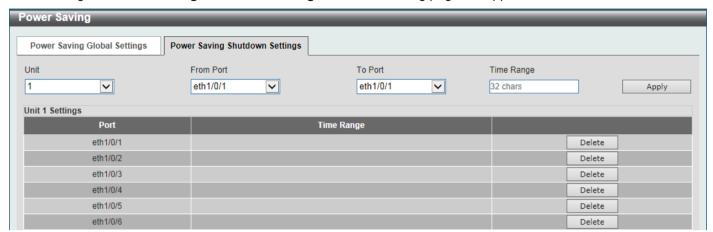
Figure 14-2 Power Saving Shutdown Settings Window
