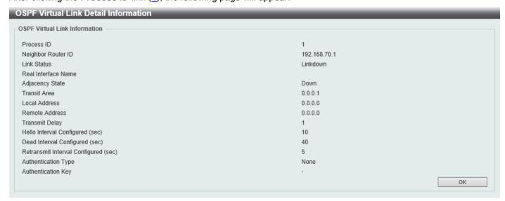
Figure 6-65 OSPFv2 Virtual Link Settings (Process ID) Window
