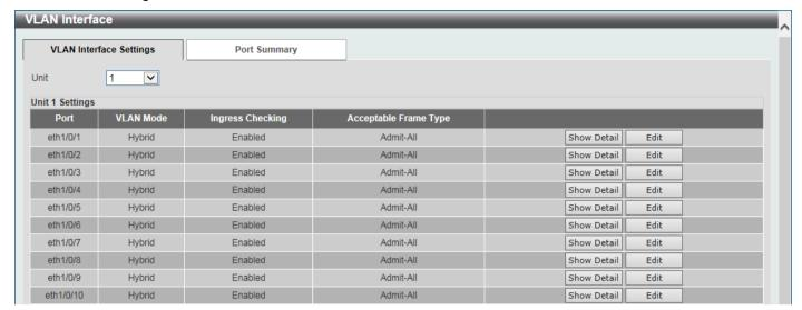
Figure 5-15 VLAN Interface Window
