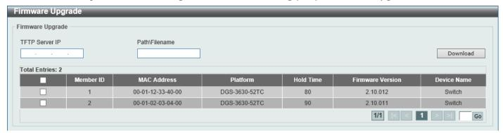
Figure 4-101 Firmware Upgrade Window
