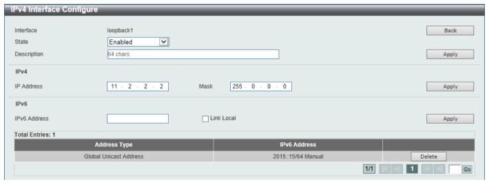
Figure 6-19 Loopback Interface (Edit) Window
