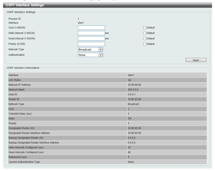
Figure 6-61 OSPFv2 Interface Settings (Show Detail) Window
