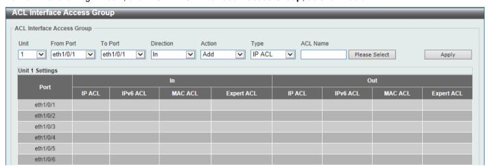
Figure 8-17 ACL Interface Access Group Window
