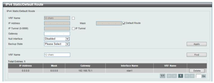
Figure 6-23 IPv4 Static/Default Route Window
