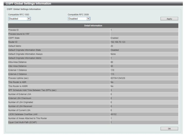
Figure 6-54 OSPFv2 Process Settings (Show Detail) Window
