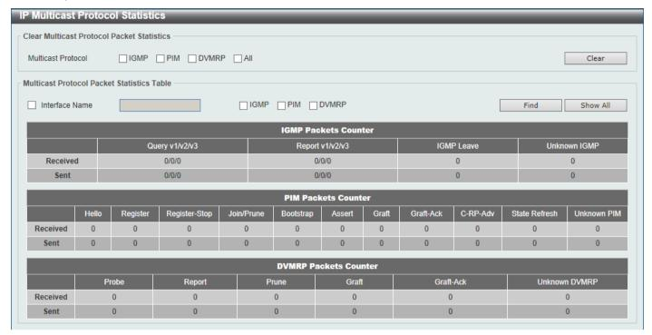
Figure 6-157 IP Multicast Protocol Statistics Window
