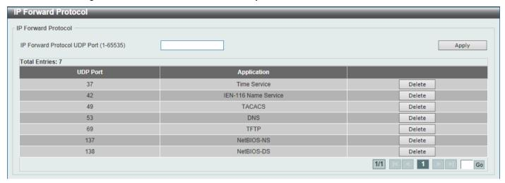
Figure 6-21 IP Forward Protocol Window
