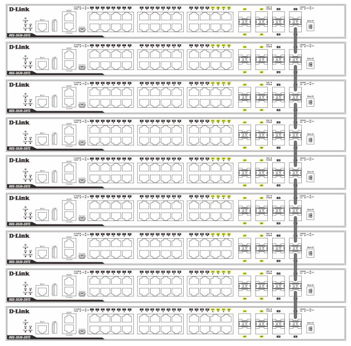
Figure 4-85 Duplex Chain stacking topology (SFP+)
