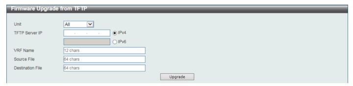
Figure 16-3 Firmware Upgrade from TFTP Window
