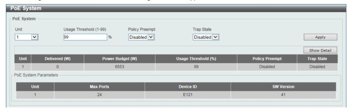
Figure 3-13 PoE System (Show Detail) Window
