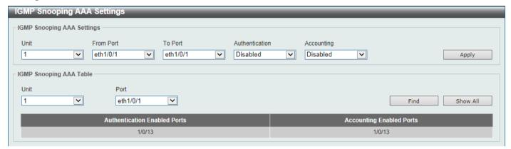
Figure 5-78 IGMP Snooping AAA Settings Window
