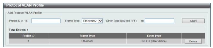
Figure 5-19 Protocol VLAN Profile Window
