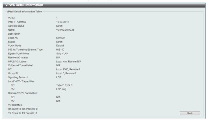
Figure 12-3 VPWS Settings (Show Detail) Window
