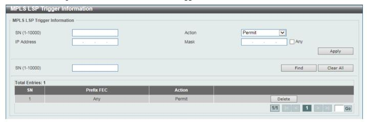
Figure 11-2 MPLS LSP Trigger Information Window
