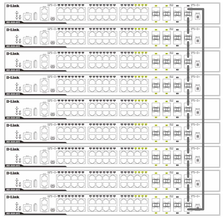
Figure 4-86 Duplex Ring stacking topology (SFP+)
