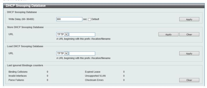
Figure 9-44 DHCP Snooping Database Window
