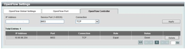
Figure 15-3 OpenFlow Controller Settings Window
