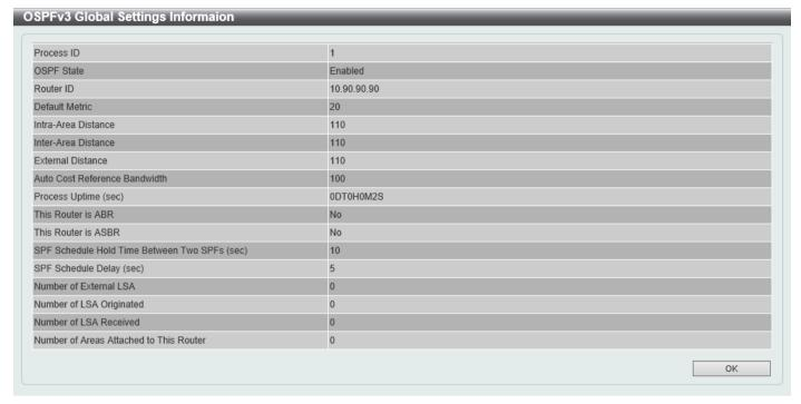
Figure 6-73 OSPFv3 Process Settings (Process ID) Window
