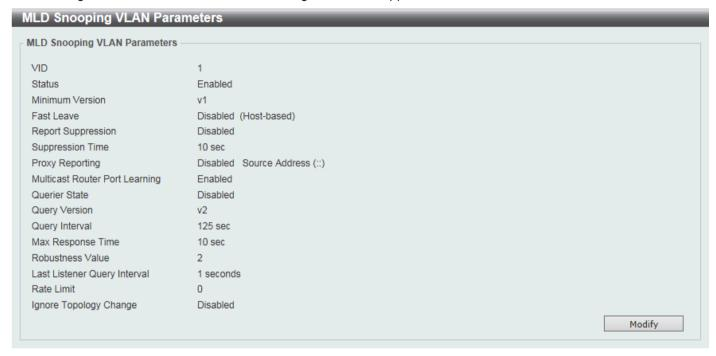
Figure 5-86 MLD Snooping Settings (Show Detail) Window
