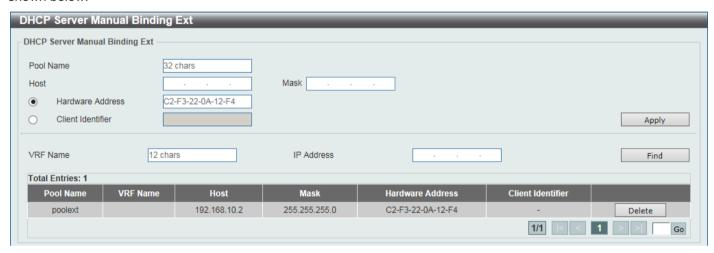
Figure 4-38 DHCP Server Manual Binding Ext Window
