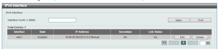
Figure 6-10 IPv4 Interface Window
