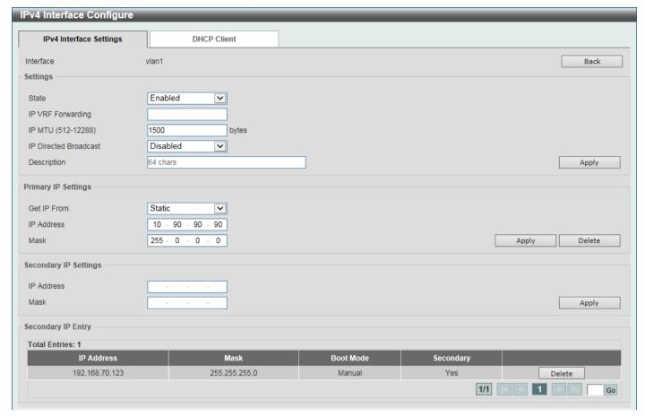
Figure 6-11 IPv4 Interface (Edit) Window
