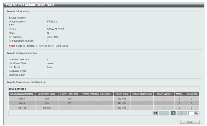
Figure 6-142 PIM for IPv6 Mroute Table (Show Detail) Window
