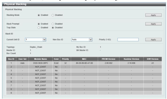
Figure 4-87 Physical Stacking Window
