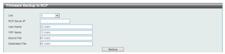
Figure 16-10 Firmware Backup to RCP Window
