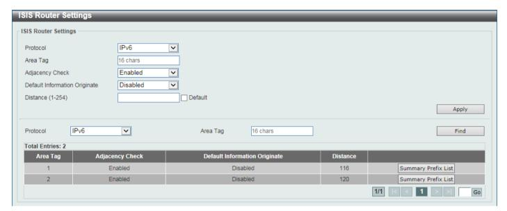
Figure 6-217 ISIS Router Settings (IPv6) Window
