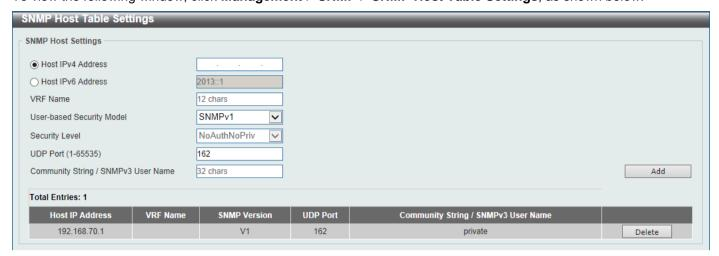
Figure 4-16 SNMP Host Table Settings Window
