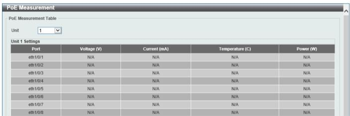
Figure 3-18 PoE Measurement Window
