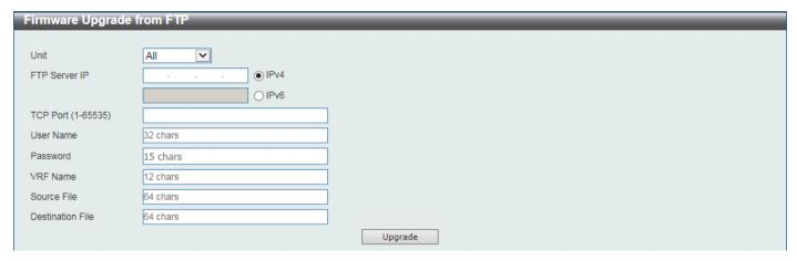
Figure 16-4 Firmware Upgrade from FTP Window
