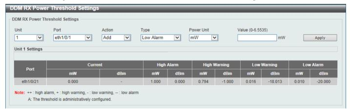
Figure 10-32 DDM RX Power Threshold Settings Window
