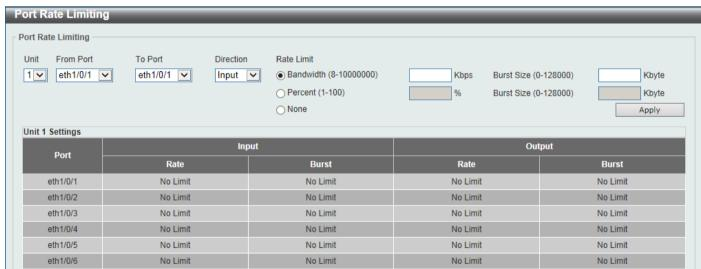
**Figure 7-5 Port Rate Limiting Window**
