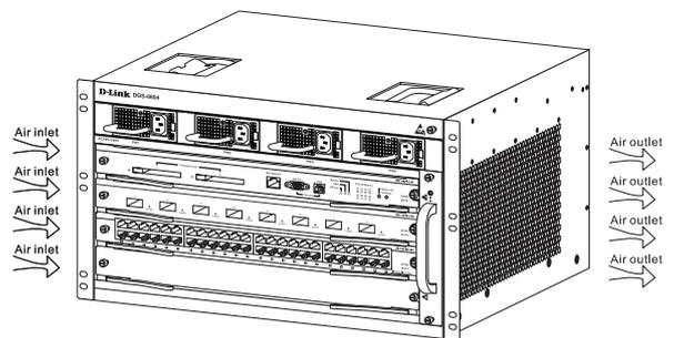
Figure 3. Ventilation of the DGS-6604
