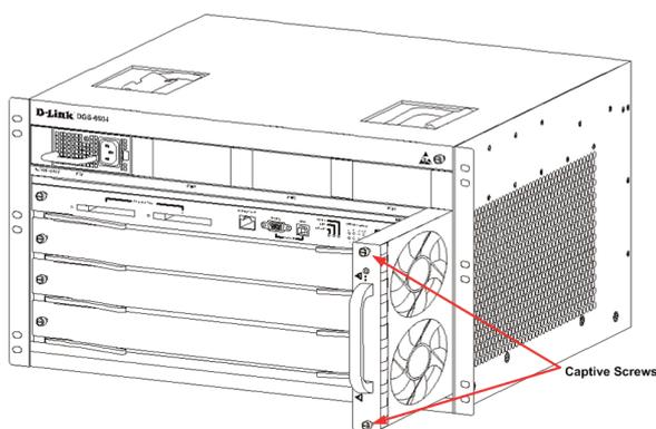
Figure 4. Installing the Fan Tray
