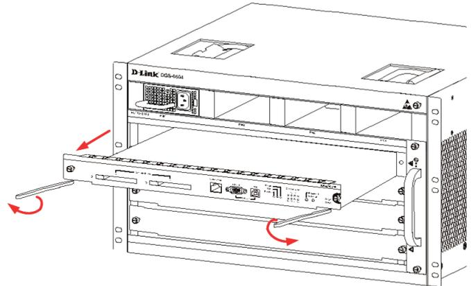
Figure 9. Removing a board from the chassis
