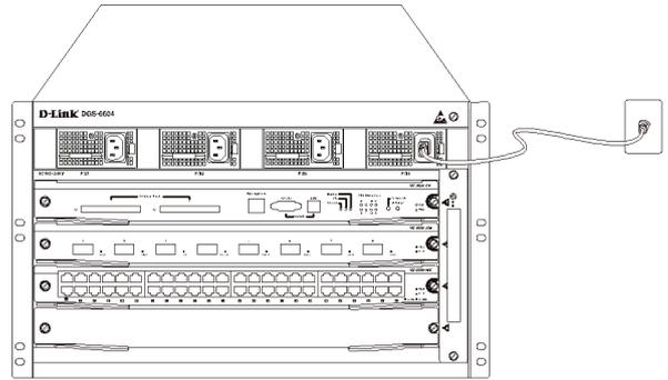
Figure 8. Connecting AC to the Power Module
