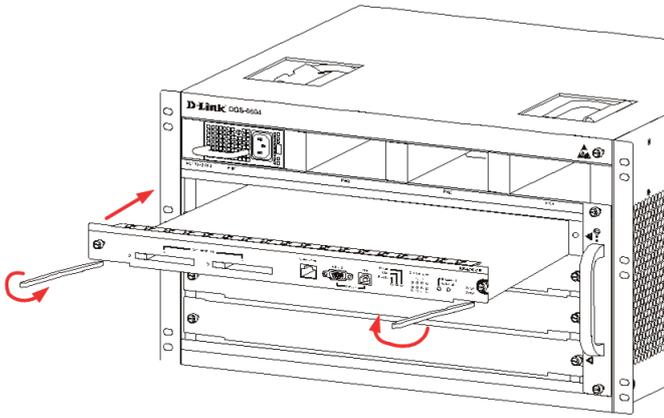
Figure 10. Installation Check
