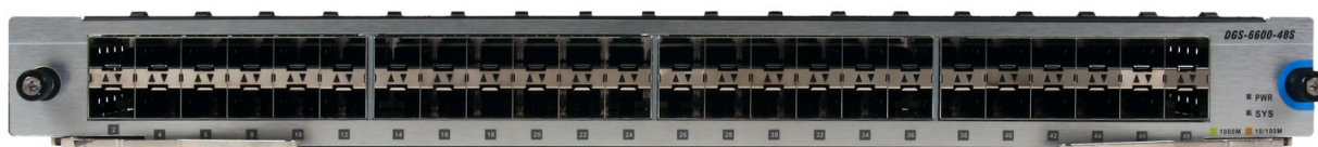
Figure 1-8 DGS-6600-48S I/O Card
