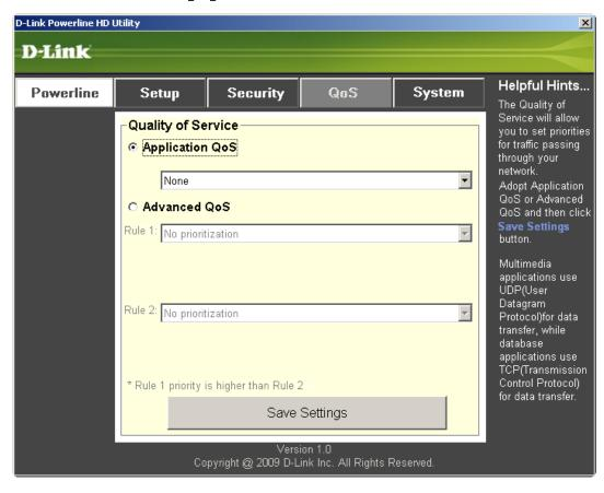
The Quality of Service (QoS) screen will allow you to set priorities for traffic passing through your network. By default all types of traffic are assigned the same priority. Multimedia applications use UDP (User Datagram Protocol) for data transfer, while database applications use TCP (Transmission Control Protocol) for data transfer.
