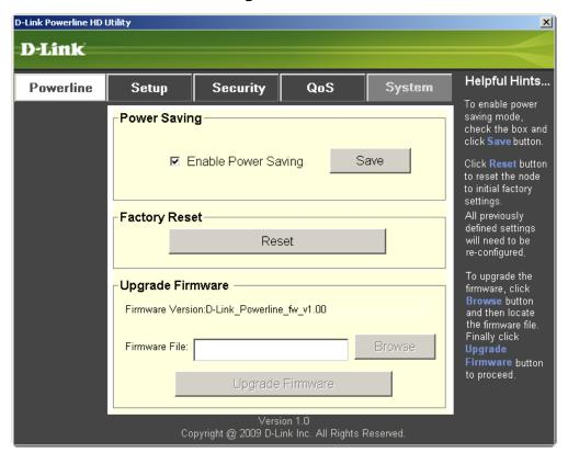
With the power saving mode enabled and the ethernet link activity being down for 15 minutes, the DHP-342 will automatically go into stand-by mode. When the master unit is in stand-by mode, the throughput LED will blink red intermittently.
