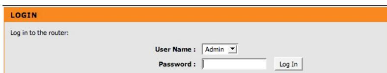
**Step 4.** If unsuccessful in accessing the router's configuration pages, please reset the router. Here is how to reset it: while the router is powered on, press and hold the Reset button for 10 sec. Release the button and wait until the router boots up (1 min). Try to log into it again.
