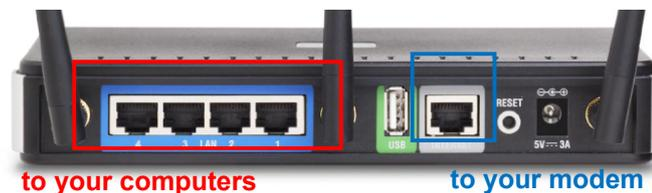
Verify physical connectivity by checking for solid link lights on the Ethernet ports of the device. If you do not get a solid link light, try using a different cable or connect to a different port on the device if possible. If the computer is turned off, the link light may not be on.
