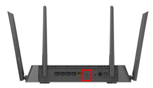
**Step 2:** The unit will reboot automatically. Once the power light stops blinking, the unit has been reset and is ready to use. **Resetting the router does not reset the firmware to the previous version, but it will change all settings back to factory defaults**.
