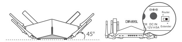
2. Connect the supplied power adapter to the DIR-895L and a power outlet.
