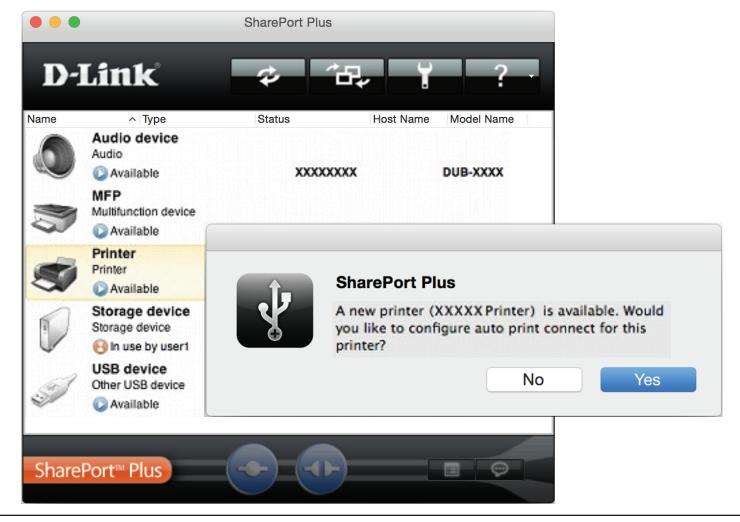
The SharePort Plus utility will automatically configure your computer to print to the printer attached to your SharePort Plus enabled DIR-895L's USB port. A green check mark ( ) indicates that the printer is connected to your Mac.
