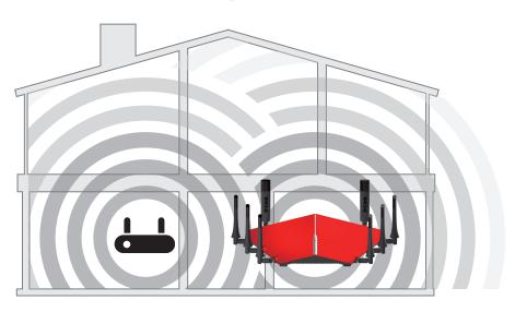
In **Media Bridge Mode**, the DIR-895L connects to your existing network wirelessly to provide connectivity to Ethernet devices. This can be useful if you cannot install Ethernet cable to your desired location or have devices which do not have wireless Ethernet. Devices connected to the DIR-895L obtain IP addresses from the existing uplink network. To use your DIR-895L as a media bridge, install it in an area where you can receive your wireless network signal.
