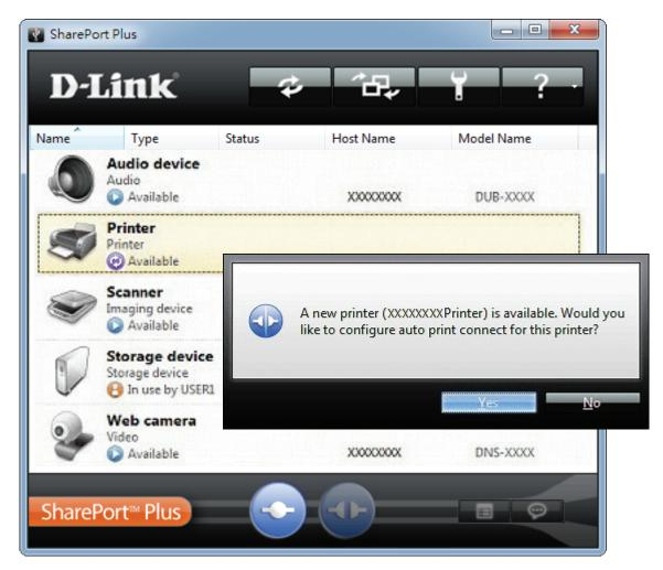
The SharePort Plus utility will automatically configure your PC to print to the printer attached to your SharePort Plus enabled DIR-895L's USB port. A green check mark ( ) indicates that the printer is connected to your PC.
