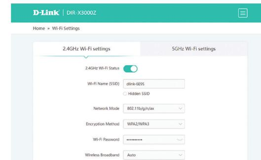
After completing the setup, the Router will restart. Reconnect to your Router's Wi-Fi using the new name and password.
