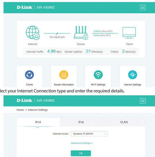
Step 4. To set up your Router's Wi-Fi, click on the Wi-Fi Settings icon. Enter the desired Wi-Fi Name and assign a secure password to your Wi-Fi.
