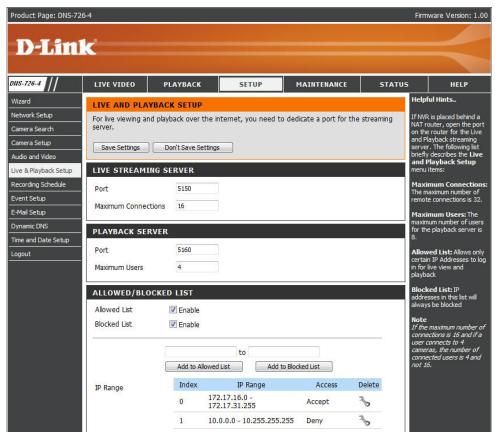
**Note:** When setting Maximum Connections in Live Streaming Server settings, 1 connection means that 1 user can connect to 1 camera only. If the maximum number of connections is 16 and if each user connects to 4 cameras, then the maximum number of connected users is 4 and not 16.
