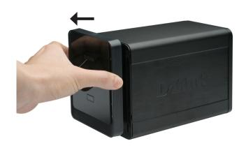
4. Insert a 3.5" SATA hard drive into an available drive bay. Make sure to align the drive connector to the SATA connector on the bottom edge inside the drive bay of the NVR. Gently push the drive in until it connects. When a drive is inserted properly, you will feel it "seat" into the connector. Some hard drives that are thin or oddly shaped may need to be guided carefully into position. If a drive is not properly seated, the LED will not illuminate once the device has been powered on.
