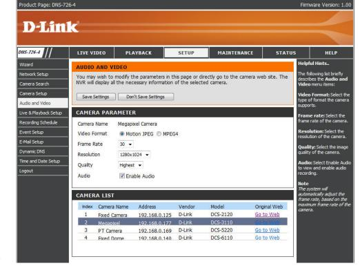
**Note:** The system will adjust the frame rate automatically based on the maximum frame rate which that camera can support.
