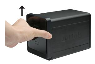
3. Once the faceplate is unlatched, pull it off the device, exposing the drive bays.
