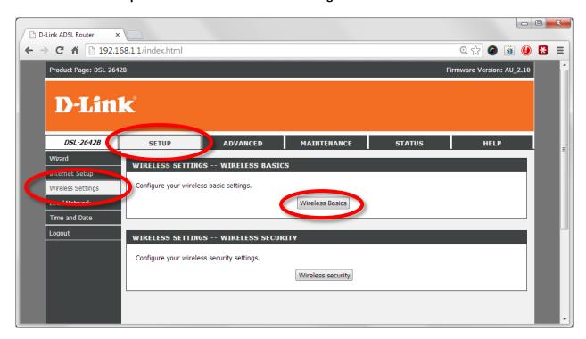
**Step 4.** In the [WIRELESS SETTING] section of the page please find the "Channel" option. Click on the drop down menu to select a channel number between 1 and 13. (Please note that although channels 12-13 are allowed in Australia/NZ some of your devices may not detect Wi-Fi on these channels due to restrictions in US).
