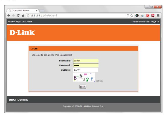
If you cannot recall the password you assigned to your modem you will need to reset the modem to factory defaults by pressing the reset button for 10 seconds. Please note that this will revert all the settings in the modem to factory settings and you will have to reconfigure it with your Internet settings and Wireless security. Make sure you have your Internet account details (given by your Internet Provider) handy.
