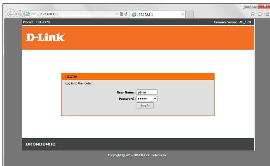
*If you cannot recall the password you assigned to your modem you will need to reset the modem to factory defaults by pressing the reset button for 10 seconds. Please note that this will revert all the settings in the modem to factory settings and you will have to reconfigure it with your Internet settings and Wireless security. Make sure you have your Internet account details (given by your Internet Provider) handy.*
