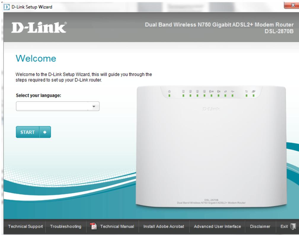
If the Install wizard does not start up automatically, you can start it up manually by double-clicking on the **DSL-2870B.exe** file in the CD-ROM Drive
